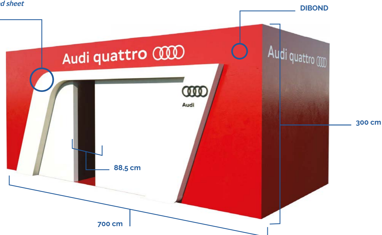
Cassonetto in ferro e lamiera zincata verniciata bianca Box in iron and white painted galvanized sheet
